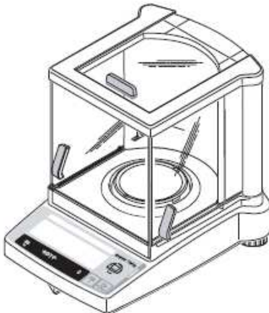
Figure 2.5: A view of the electronic balance to be used in your experiment.
