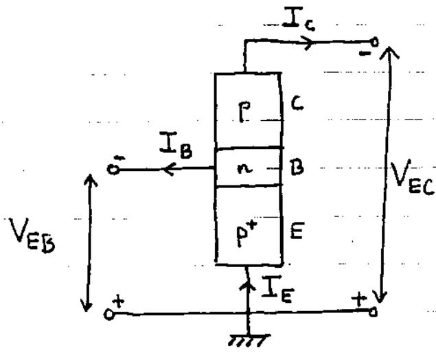
$$\begin{aligned} I_c &= \alpha_0 I_e + I_{CBO} \\ &= \alpha_0 (I_B + I_c) + I_{CBO} \end{aligned}$$
