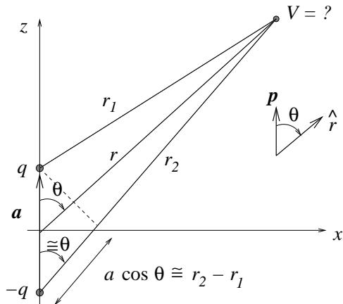
$$\begin{aligned} V(r, \theta) &= \frac{q}{4\pi\epsilon_0} \left( \frac{1}{r_1} - \frac{1}{r_2} \right) \\ &= \frac{q}{4\pi\epsilon_0} \cdot \frac{r_2 - r_1}{r_1 r_2} \\ &\simeq \frac{q}{4\pi\epsilon_0} \cdot \frac{a \cos \theta}{r^2} \end{aligned}$$
