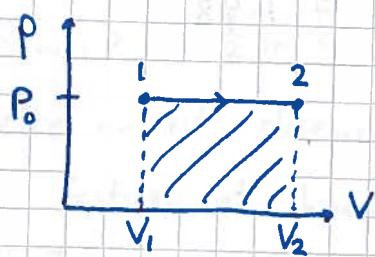
$$W = \int_1^2 dW = P_0 \int_{V_1}^{V_2} dV = P_0 (V_2 - V_1)$$
