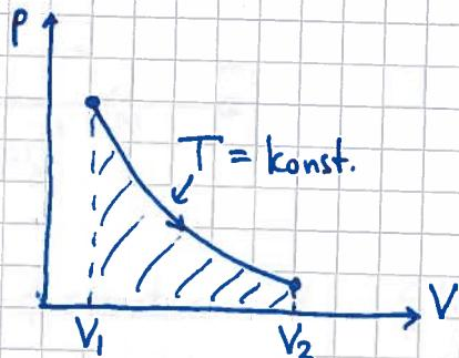
$$\begin{aligned} p(V) &= Nk_B T / V \\ \Rightarrow W &= Nk_B T \int_{V_1}^{V_2} \frac{dV}{V} = Nk_B T \ln \frac{V_2}{V_1} \end{aligned}$$
