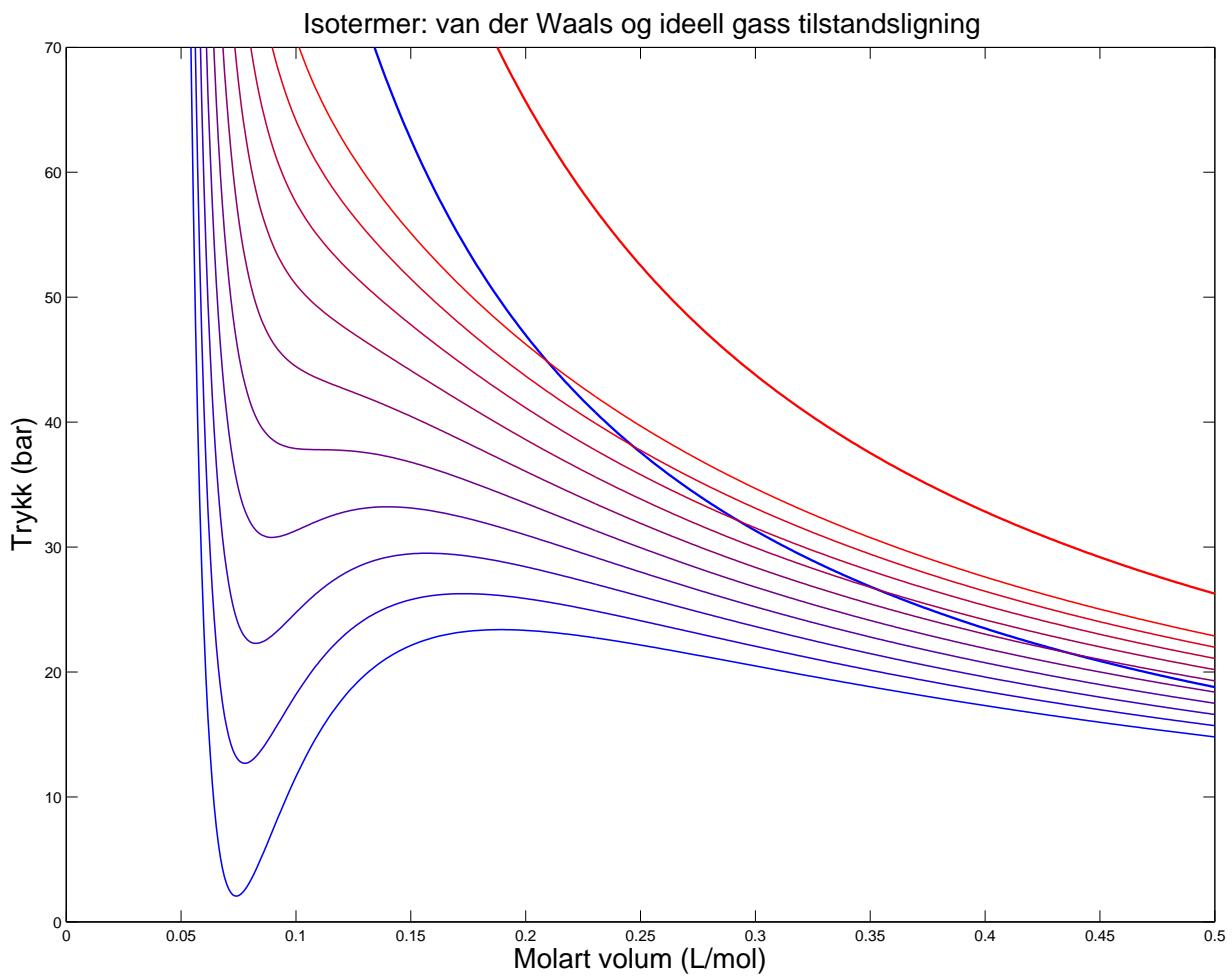
Figur 2: Isotermer for van der Waals tilstandslingning (tynne kurver) og for ideell gass (tykke kurver). Temperaturer, van der Waals: 113, 118, 123, 128, 133, 138, 143, 148, 153, 158 K. Temperaturer, ideell gass: 113, 158 K.
