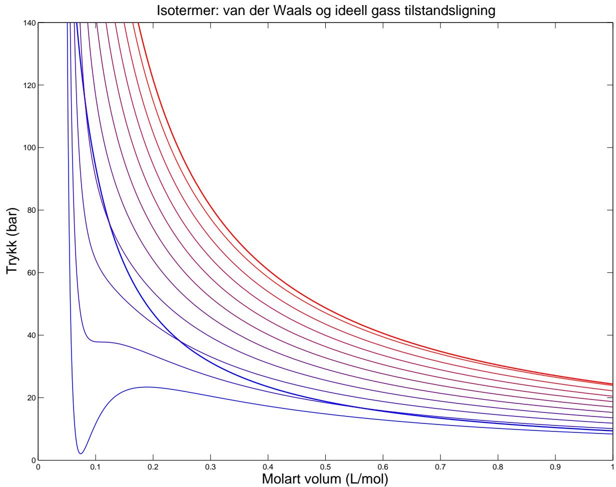
Figur 1: Isotermmer for van der Waals tilstandslegning (tynne kurver) og for ideell gass (tykke kurver). Temperaturer, van der Waals: 113, 133, 153, 173, 193, 213, 233, 253, 273, 293 K. Temperaturer, ideell gass: 113, 293 K.
