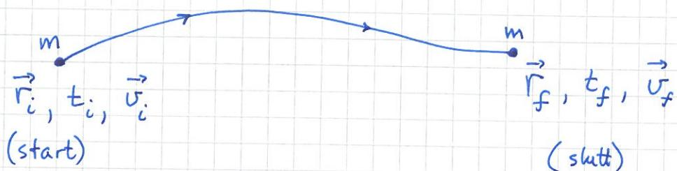
$$W = \int_{\vec{r}_i}^{\vec{r}_f} \vec{F} \cdot d\vec{r} = \int_{t_i}^{t_f} m \frac{d\vec{v}}{dt} \cdot \vec{v} dt = m \int_{t_i}^{t_f} \frac{d}{dt} \left( \frac{1}{2} \vec{v} \cdot \vec{v} \right) dt = \frac{1}{2} m v_f^2 - \frac{1}{2} m v_i^2$$
