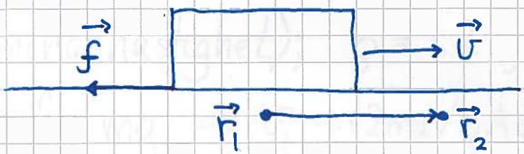
$$W_f = \int_{\vec{r}_1}^{\vec{r}_2} \vec{f} \cdot d\vec{r} < 0 \quad \text{da } \vec{f} \text{ alltid rettet mot } d\vec{r}$$
