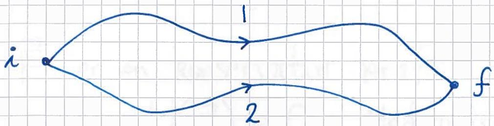
$$0 = \oint \vec{F} \cdot d\vec{r} = \left\{ \int_i^f \vec{F} \cdot d\vec{r} \right\}_1 + \left\{ \int_f^i \vec{F} \cdot d\vec{r} \right\}_2 \\ = W_1 - W_2 \\ \Rightarrow W_1 = W_2 \quad (\text{qed})$$
