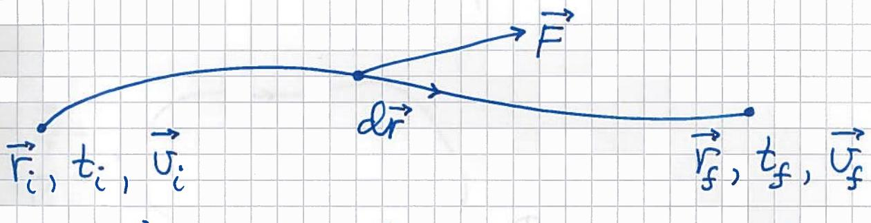
$$W = \int_{\vec{r}_i}^{\vec{r}_f} \vec{F} \cdot d\vec{r} = \int_i^f m \frac{d\vec{v}}{dt} \cdot \vec{v} dt = m \int_i^f \vec{v} \cdot d\vec{v}$$
