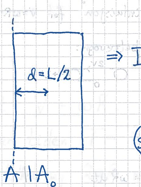
$$\begin{aligned} I &= I_0 + M \cdot \left(\frac{L}{2}\right)^2 \\ &= \frac{1}{3} M L^2 \end{aligned}$$
