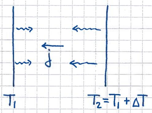
$$j = \sigma (T_2^4 - T_1^4) = \sigma (T_2^2 + T_1^2)(T_2^2 - T_1^2)$$
