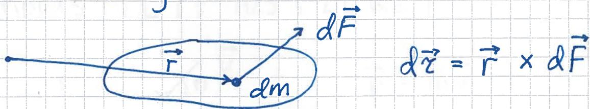
$$\vec{L} = \int d\vec{L} = \int \vec{r} \times d\vec{F} = \text{totalt dreiemoment p\u00e5 systemet}$$
