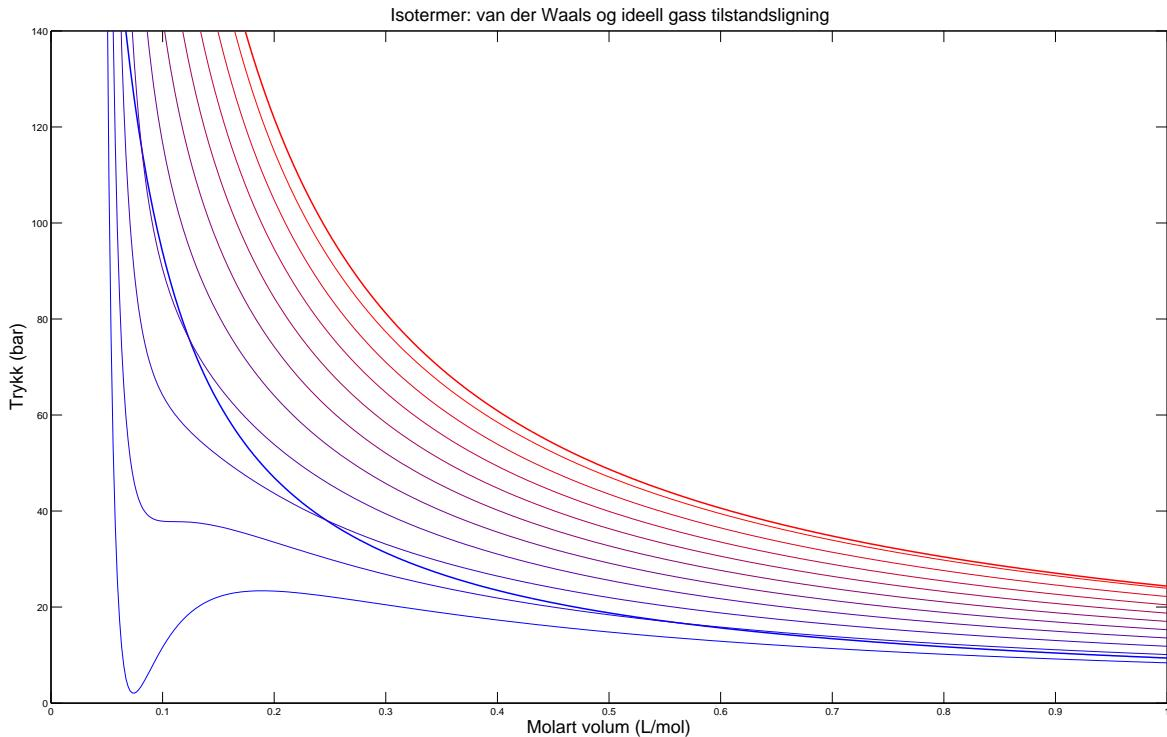
Figur 1: Isotermer for van der Waals tilstandslingning (tynne kurver) og for ideell gass (tykke kurver). Temperaturer, van der Waals: 113, 133, 153, 173, 193, 213, 233, 253, 273, 293 K. Temperaturer, ideell gass: 113, 293 K.
