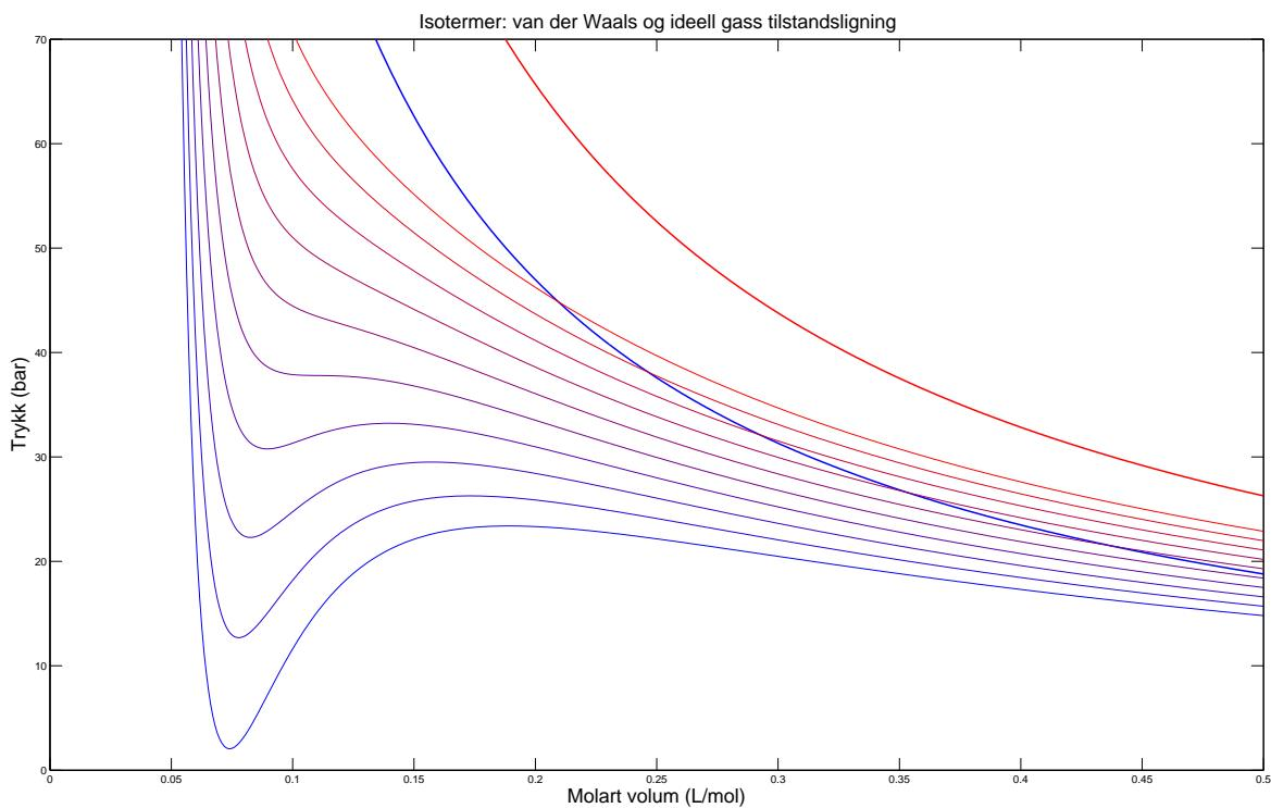
Figur 2: Isotermer for van der Waals tilstandslikning (tynne kurver) og for ideell gass (tykke kurver). Temperaturer, van der Waals: 113, 118, 123, 128, 133, 138, 143, 148, 153, 158 K. Temperaturer, ideell gass: 113, 158 K.
