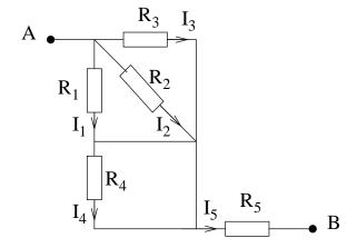
a) Determine the total resistance R between the points A and B, i.e.: Determine the resistance R in the equivalent circuit in the following figure:
