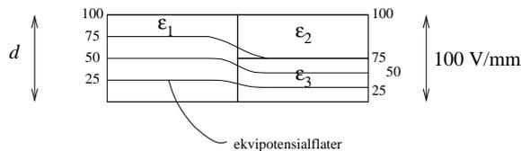
From the shape of the sketched equipotential surfaces, we see that the electric field must have a horizontal component in the vicinity of the vertical midplane, since  $\mathbf{E} = -\nabla V$  is always perpendicular to the equipotential surfaces.
