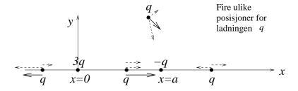
a) The point charge q is in equilibrium if there is no force acting on it. Here, two forces are acting, one repulsive due to the charge 3q and one attractive due to -q. These two may cancel each other, but only if they point in opposite directions. This is not possible if q is located off the x axis, e.g. as in the figure above. (Here, dashed arrows denote partial forces and solid arrows the total force.) Hence, any equilibrium position must be on the x axis.
