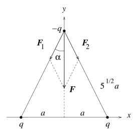
The third charge is supposed to be equally far from the two others, on the positive y axis. Pytagoras then yields a position  $y = \sqrt{(\sqrt{5}a)^2 - a^2} = 2a$  for the third charge.
