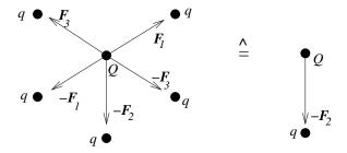
It is then immediately clear that the net force on Q equals the force due to the removed charge, but with opposite sign, i.e.,  $-\mathbf{F}_2$ .
