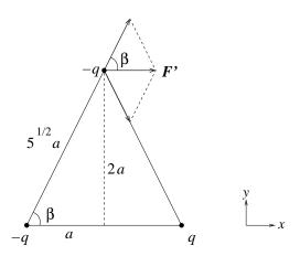
We see from the figure that the total force F' points in the positive x direction. The x component of each of the partial forces is found by multiplying with  $\cos \beta = 1/\sqrt{5}$ . Hence we see that F' must be half as big as F, i.e.,
