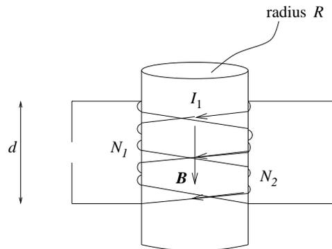
The figure shows two solenoids 1 and 2 that are both wound onto the same cylinder of radius  $R$ . We assume that the cylinder has magnetic properties as vacuum, i.e., we assume there is no magnetization of the cylinder. Solenoid 1 has  $N_1$  windings, solenoid 2 has  $N_2$  windings. Both solenoids are wound onto a length  $d$  of the cylinder, which is (approximately infinitely) long compared to the radius of the cylinder. (So the figure is only qualitatively correct...!) You
