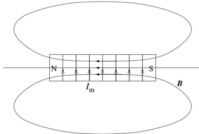
b) Let us imagine cylinder formed bar magnets. Such a magnet can then be viewed as a current carrying cylindrical "shell", alternatively closely spaced current carrying rings. We look at the magnetic force acting on such a ring in the magnetic field from the other bar magnet:
