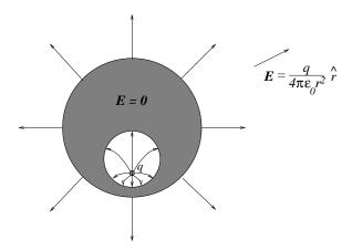
We have chosen to draw 8 field lines pr charge q. All 8 field lines starting on the point charge must terminate on the surface of the cavity, and in such a way that they are perpendicular to the surface. (Electric field always normal to a metal surface!) Inside the conductor, E=0, so here we have no field lines. On the outer surface, we have a charge q uniformly distributed, so here we have again 8 field lines, directed radially outwards.
