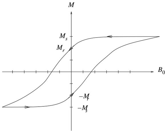
The *shape* of the hysteresis curve will tell you whether you have a so called "hard magnet" (i.e. a permanent magnet) or a "soft magnet" (for example a piece of steel):
