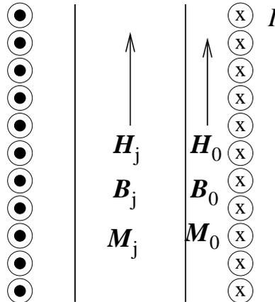
A cylindrical iron rod with relative permeability  $\mu_r = 2000$  is placed coaxially inside a solenoid, but fills only partially the volume inside the solenoid. The solenoid has a winding density (i.e., windings pr unit length)  $n = 2000 \text{ m}^{-1}$  and the current in the solenoid wire is  $I = 3 \text{ A}$ . We assume that both the solenoid and the iron rod are sufficiently long that we may neglect edge effects.
