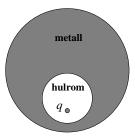
What can you then say about the distribution of (free) charge in the metal sphere, given that we have electrostatic (equilibrium) conditions? [Hint 1: What is the electric field inside the metal? Hint 2: Use Gauss' law to support your arguments.]
