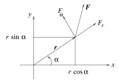
Further, we know that the force  $\mathbf{F}$  may be derived from the potential energy U using the gradient operator:  $\mathbf{F} = -\nabla U$ . In polar coordinates  $(r, \alpha)$ , we have
