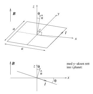
The orientation of the current loop is defined through the angle  $\theta$  between the z-axis and the surface normal  $\hat{n}$ . (Positive  $\theta$  counterclockwise, as shown in the figure.)
