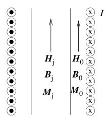
A cylindrical iron rod with relative permeability  $\mu_r = 2000$  is placed coaxially inside a solenoid, but fills only partially the volume inside the solenoid. The solenoid has a winding density (i.e., windings pr unit length)  $n = 2000 \text{ m}^{-1}$  and the current in the solenoid wire is I = 3 A. We assume that both the solenoid and the iron rod are sufficiently long that we may neglect edge effects.
