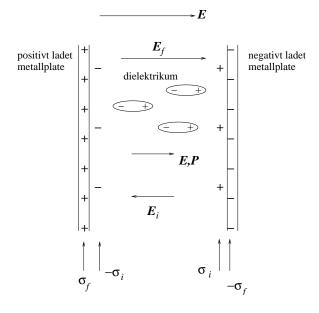
Free charge pr unit area on the metal plates:  $\sigma_f$
