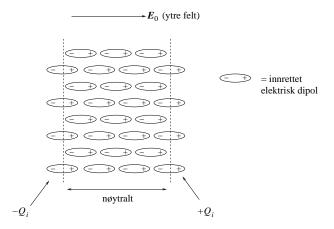
$\pm Q_i$  = net induced charge on the surface of the insulator.
