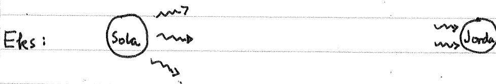
$$P_{\text{rad}} \sim 10^{-6} \text{ N/m}^2 \ll P_{\text{atm}} = 10^5 \text{ N/m}^2$$
