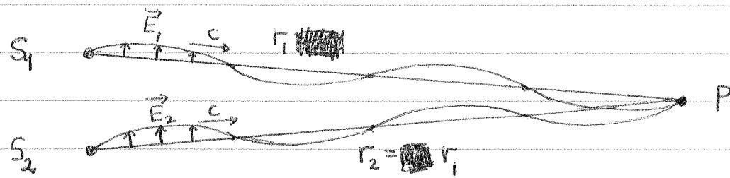
$$\vec{E}_p = \vec{E}_{1p} + \vec{E}_{2p} = \vec{E}_{10} \cos(\vec{k}_1 \cdot \vec{r}_1 - wt) + \vec{E}_{20} \cos(\vec{k}_2 \cdot \vec{r}_2 - wt)$$
