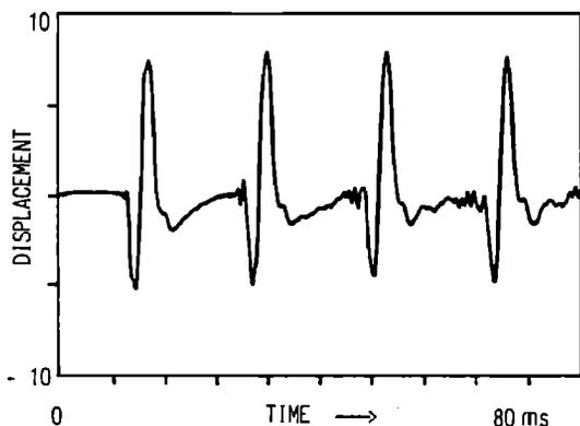
FIG. 8. A trace of the perpendicular-to-soundboard displacement of an  $A_1$  (55-Hz) string in time, showing the first four initial pulses monitored approximately 10 cm from the bridge. The unit of the displacement scale is arbitrary.
