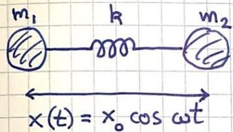
$$E^{\text{vib}} = E_k^{\text{vib}} + E_p^{\text{vib}} = \frac{1}{2} \mu \dot{x}^2 + \frac{1}{2} k x^2$$
