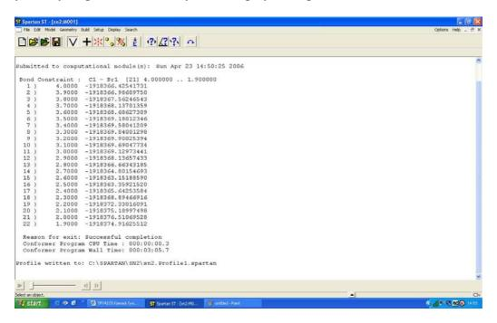
Here, you notice that a new file, sn2.Profile1.spartan, has been created. This file contains the results of all the 22 geometry optimizations, i.e., geometries and corresponding energies, and also the basis for analyzing the results in terms of graphs. Choose File – Close and open the file sn2.Profile1.spartan. "Play" the reaction with the "molecule player" in the lower left corner.
