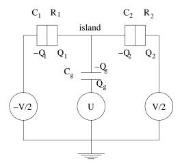
The tunneling junctions both have a large resistance compared to the quantum of resistance  $R_Q = h/e^2$ . The island has a net charge q = -ne, corresponding to n "extra" electrons. Bias voltages  $\pm V/2$  are applied to the tunneling junctions, as illustrated in the figure.
