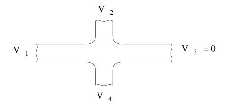
We choose  $V_3 = 0$ . According to Büttiker and Landauer, the current in terminal  $\alpha$  is
