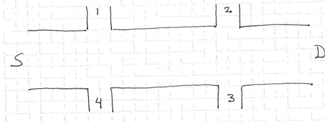
1-4 : Ohmic contacts; for voltage or current measurements
