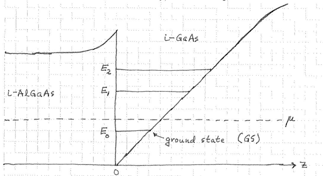
Quantized movement in  $z$ -direction, periodic potential in  $xy$  plane.
