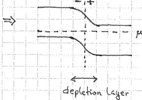
$$\text{Diode: } I(V) = I_0 \left\{ e^{\frac{eV}{k_B T}} + 1 \right\}$$
