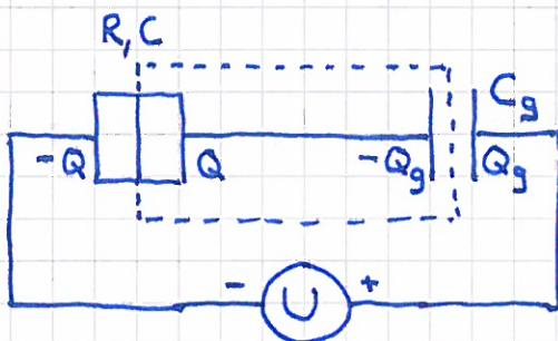
[ ] = electron box, island with quantized net charge
