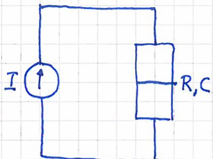
$$Q(t) = C \cdot V(t) = \int_0^t I dt' + \Delta Q_{\text{tunnel}}$$
