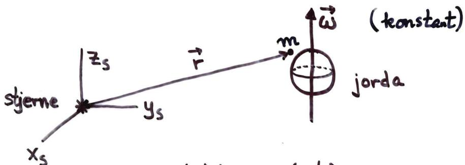
$$\left(\frac{d}{dt}\right)_s = \left(\frac{d}{dt}\right)_r + \vec{\omega} \times$$
