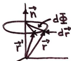
$$d\vec{r} = \vec{r} \times \vec{n} d\Phi \quad (\text{se s. 32})$$
