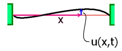
A "cable" in this context implies no stiffness; the restoring force comes from the fact that the cable is in tension (assumed constant) T.
